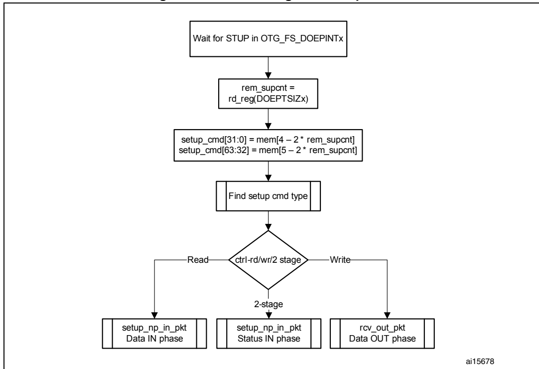
Figure 425. Processing a SETUP packet
