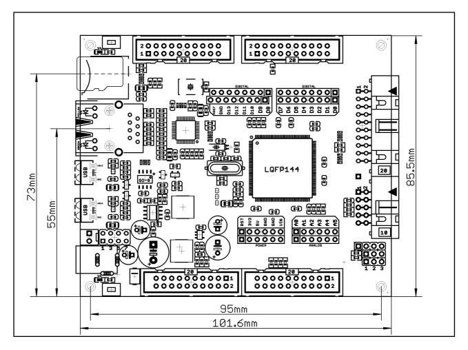
The three highest elements on the board in order from the tallest to the shortest are: capacitor C50 – 17.2mm (0.677") over the pcb; LAN connector – 13.6mm (0.535"); capacitors C42 and C48 – 11.5mm (0.453").
